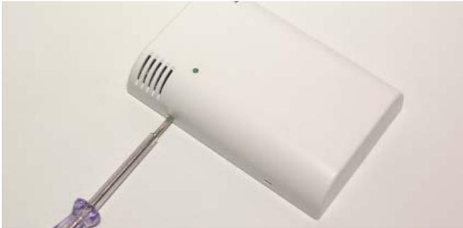
Set the thermostat GSM side of the original thermostat. It is important that the place of installation there is a good GSM signal. The device provides an internal antenna that is suitable for most applications. Otherwise you can connect an external antenna with cable stylus supplied. With a screwdriver press the tabs and remove the back of the container.
