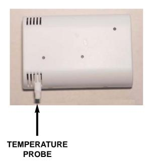
Press the cover on the base until it clicks. Place the device with the temperature probe facing downward.
