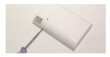
Set the thermostat GSM side of the original thermostat. It 'important that the place of installation there is a good GSM signal. The device provides an internal antenna that is suitable for most applications. Otherwise you can connect an external antenna with cable stylus supplied. With a screwdriver press the tabs and remove the back of the container.
