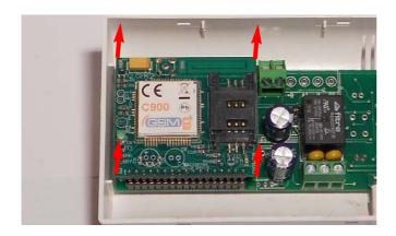
Gently pull up the tab on which is the GSM modem and the SIM holder to remove it from the base.
