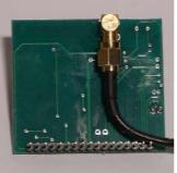
Under this tab is mounted a connector type SMA-F. Screw in the latter SMA-M of the rod antenna.
