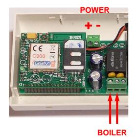
Insert the SIM in its connector: push the connector to the left, lift the cover, insert the SIM with the contacts facing down, lower the tongue and move it to the right until it clicks.
