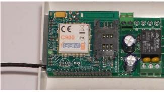
With a wire cutter to cut laterally the container so as to allow the output of the antenna cable.
